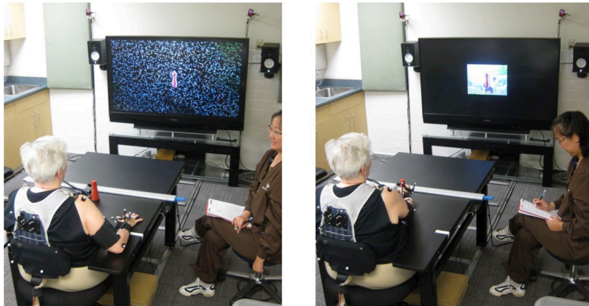
Figure 1. AMRR System. As the stroke survivor performs a reach, her movements are mapped to the image on the screen (e.g. the picture comes into focus when the reach is complete) and sounds playing from the speakers. The movements are measured by data from markers on her hand, arm and body, collected by OptiTrack cameras (two shown above the screen). The therapist is present to aid in understanding the feedback and to provide additional instruction.
